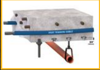
Post Tension Concrete
